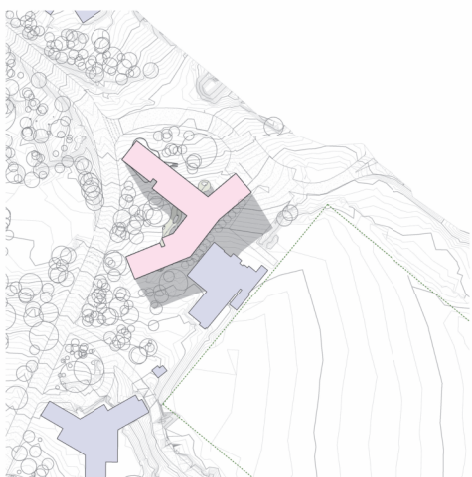
5 SHADOW DIAGRAM - SEPTEMBER 22 - 3PM SCALE 1:500
