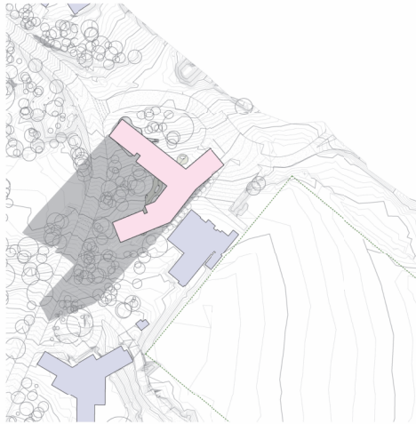
1. SHADOW DIAGRAM - JUNE 21 - 9AM Scale: 1:100
