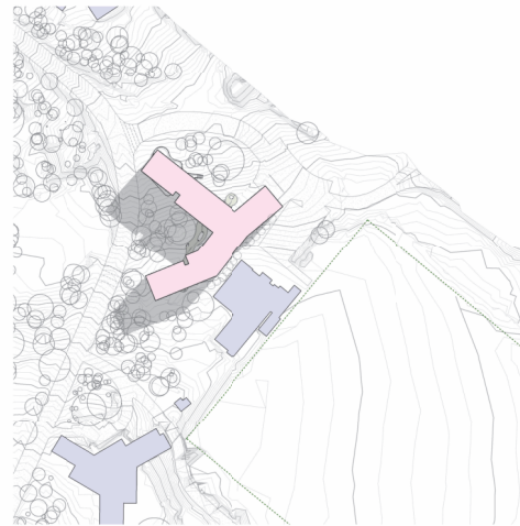
2 SHADOW DIAGRAM - SEPTEMBER 22 - 10AM SCALE 1:500
