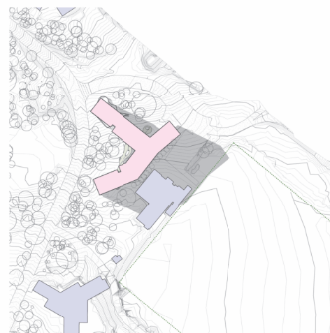
7 SHADOW DIAGRAM - SEPTEMBER 22 - 3PM SCALE 1:500
